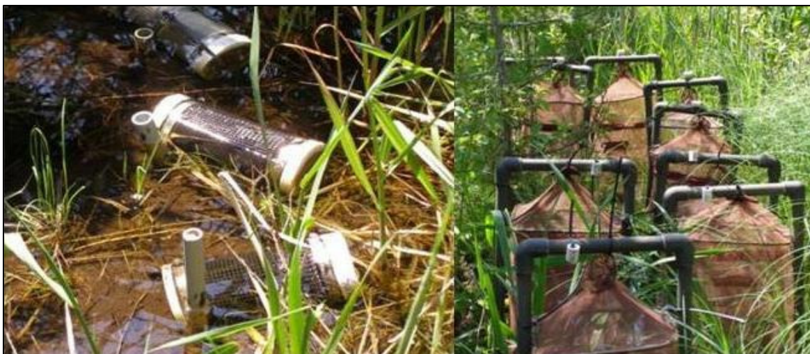
Figure 3: Standardized small growth (“S-cages”) (left photo) and emergence cage (“E-cages”) (right photo) designs for housing larvae in the field, developed in 2006.
